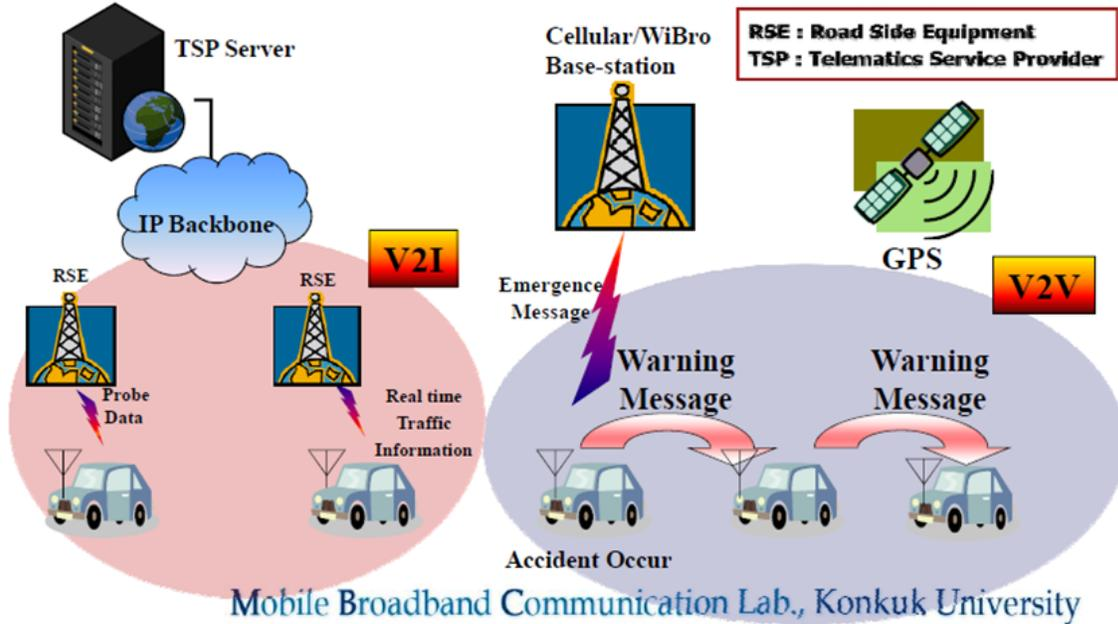
Figure 3-2: Example of Vehicular Communications
